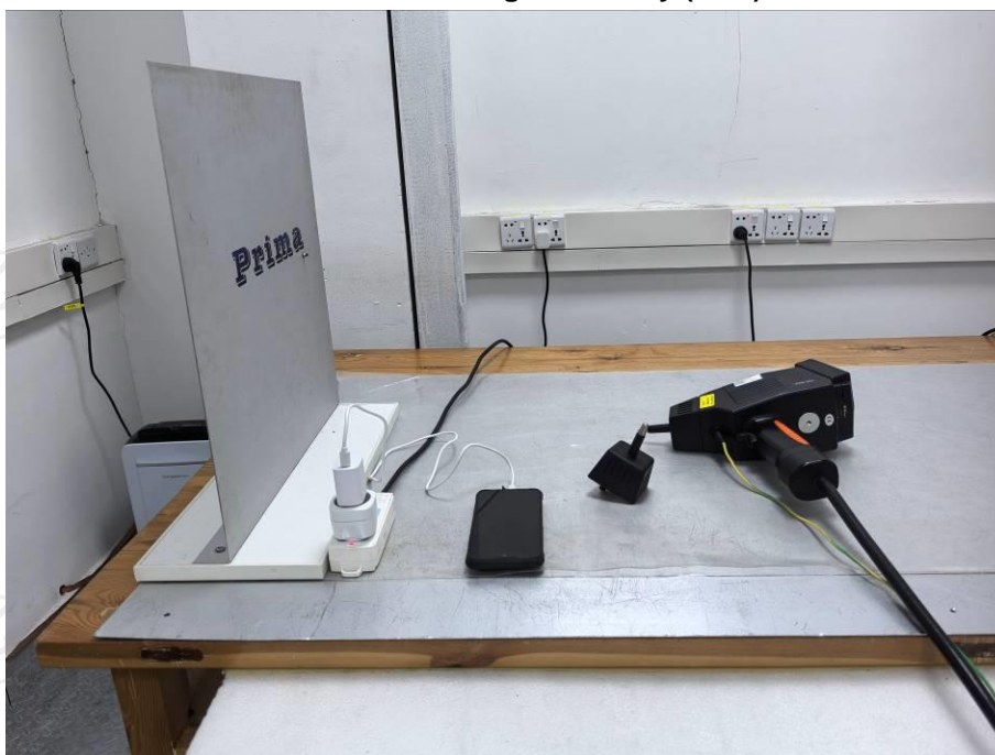
Electrostatic discharge immunity (ESD) test view
