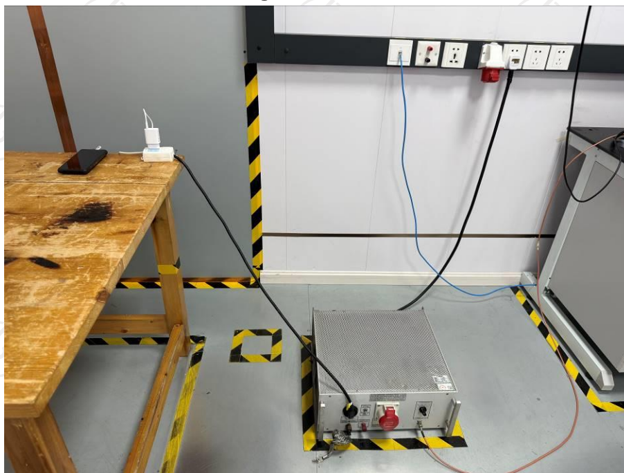
Disturbance voltage at mains terminals test view
